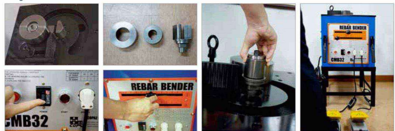
1. Turn on power 2. Adjust bending angle 3. Adjust bending radius 4. Press foot switch
